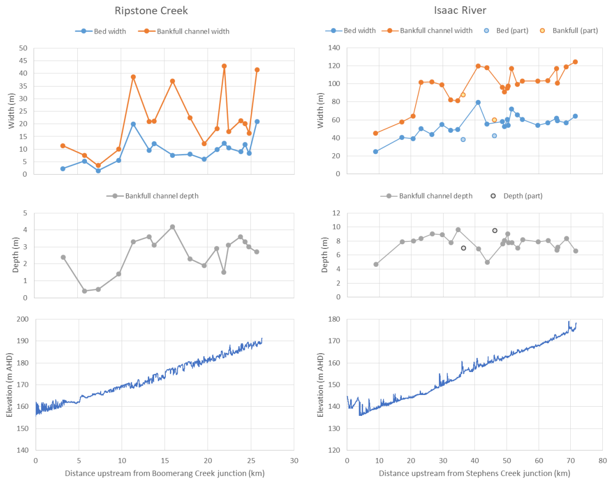
Figure 31. Downstream pattern of field-measured channel width and depth, and DEM-derived elevation of Isaac River and Ripstone Creek in the Study Area. Elevation is along 1:100,000 watercourse lines at 5 m intervals from 5 × 5 m DEM. Substantial islands were present at two sites labelled 'part' on Isaac River. Data refer to the main channel only.
