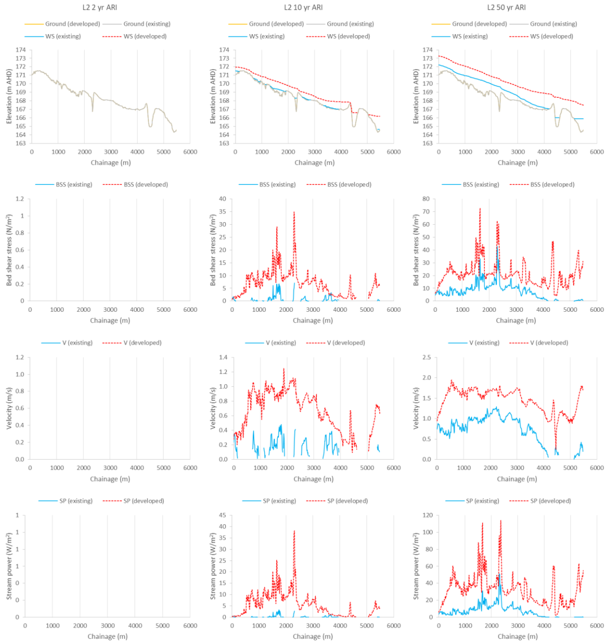
Figure 44. Long-profile 2D hydraulic character for 2 year, 10 year and 50 year ARI events. Note that Y-axis scales vary between flow scenarios.
